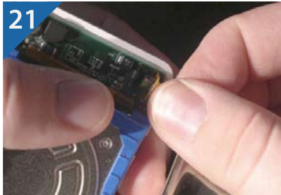
21. Reattach the back case as shown
