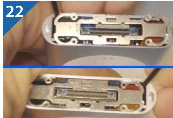
22. Insert the metal bracket (adhesive side out) back into the grooves on the bottom. Repeat the initial step of prying down on each corner to lock the bracket back into the top grooves.
