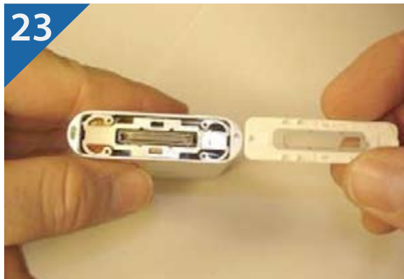
23. Reattach the plastic cover. Take note that it must be inserted in a specific way. Line up the cut out piece on the plastic cover with the metal clips on the connector inside the chassis.
