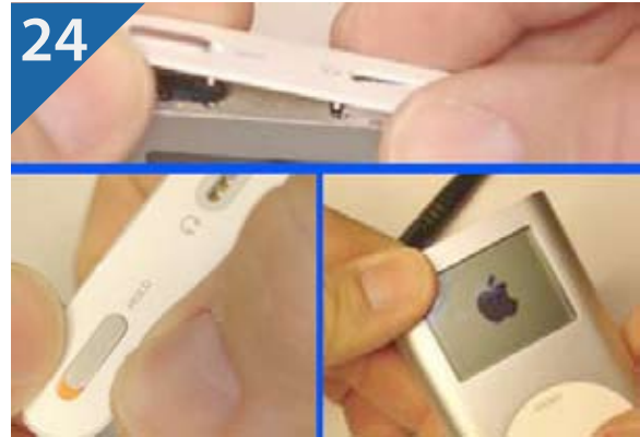
24. Reattach the screws to the top of the chassis and insert the plastic cover w/ hold switch, lining it up with the hold switch in the logic board. Turn the hold switch off and the iPod on. You're done!
