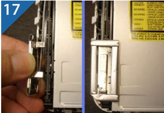
17. Locate the smaller antenna board (Bluetooth) and insert the metal fin in between the black plastic chassis and the optical drive (there is a small slot for this purpose).
