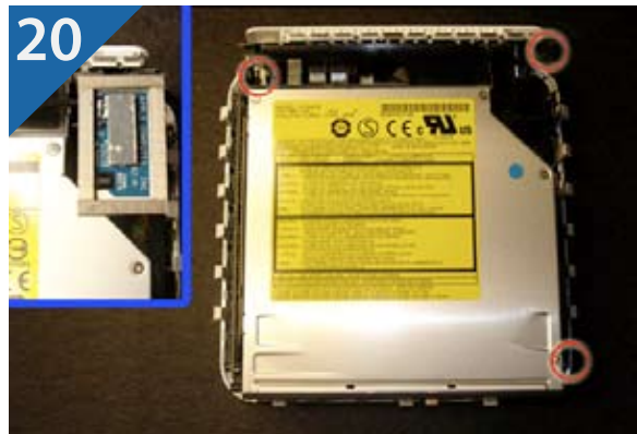
20. Reinsert the three screws for the chassis. Note: you might need to temporarily lift up the 802.11 b/g antenna to gain access to the screw hole. Simply reattach when done.
