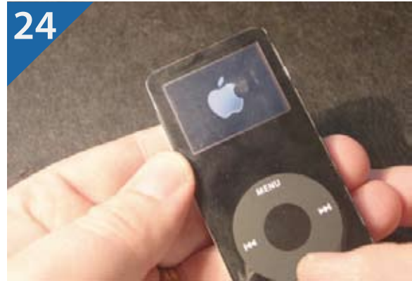
24. Press the play/pause button and/or the center select button to turn your iPod back on. You're done!
